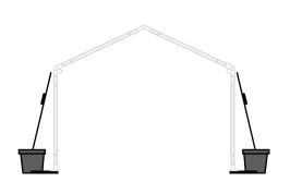
Attach Giffy Plates to underside of barrel using hardware kits; Install to the bottom of each leg
