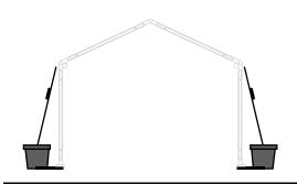
Attach Giffy Plates to underside of barrel using hardware kits; Install to the bottom of each leg
