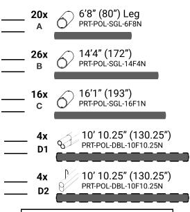
Note: Poles D1 and D2 connect together to make Pole D. See Double Tube Set Up Instructions for futher detail.
