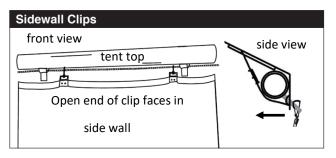
Attach the first clip onto the sidewall rope and then walk slowly, attaching every third clip. Once every third clip is attached and the sidewall is hanging in the desired location go back and attach the remaining clips.
