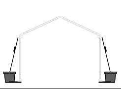
Attach Giffy Plates to underside of barrel using hardware kits; Install to the bottom of each leg
