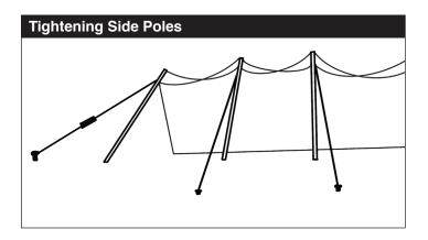
Raise poles until slightly less than perpendicular.
