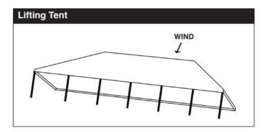
13. Attach all leg poles to the lifted side making sure the pin <u>BPN</u> is installed from the outside in.
