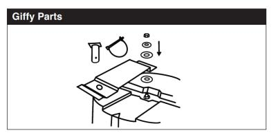
2. Assemble the hardware for the Giffy barrel using the following sequence:
