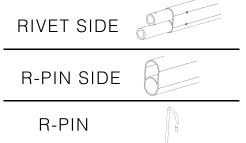
ENSURE THAT THE DOUBLE TUBE IS LINED UP PROPERLY WITH THE R-PIN HOLE FACING UP
